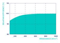
Typical module performance under low irradiance conditions in comparison to STC conditions ( $25 \,^\circ$ C, 1000 W/m<sup>2</sup>).
